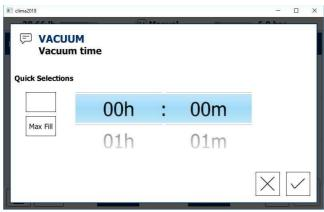
Fig. 19: Vacuum time adjustment
