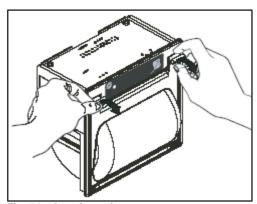
Fig. 31: Opening printer
