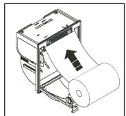
Fig. 32: Installing new paper roll
