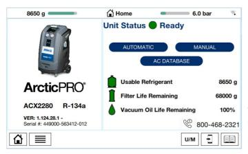
To select a function in the menu, press the text name of the function and the selection occurs when finger is released. The selected entry is highlighted with a different color (from blue to gray) and the menu screen pages changes.
