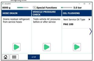
Fig. 23: Vehicle pressure check
