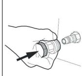
Fig. 9: Fastening quick release coupling
